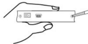
4. Replace and tighten the two screws to complete the procedure.
