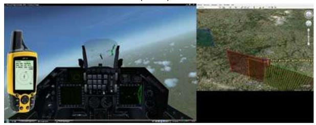
When you are running in realtime mode, traffic can also be displayed. To do that, switch the TCAS on (set the TCAS in a mode which is not OFF). You will see all the aircraft within the selected range with their callsign and relative altitude. The predicted paths of these planes have got a color code, see the color codes above. Realtime must be enabled off course, see Realtime flightlogging for more information.
