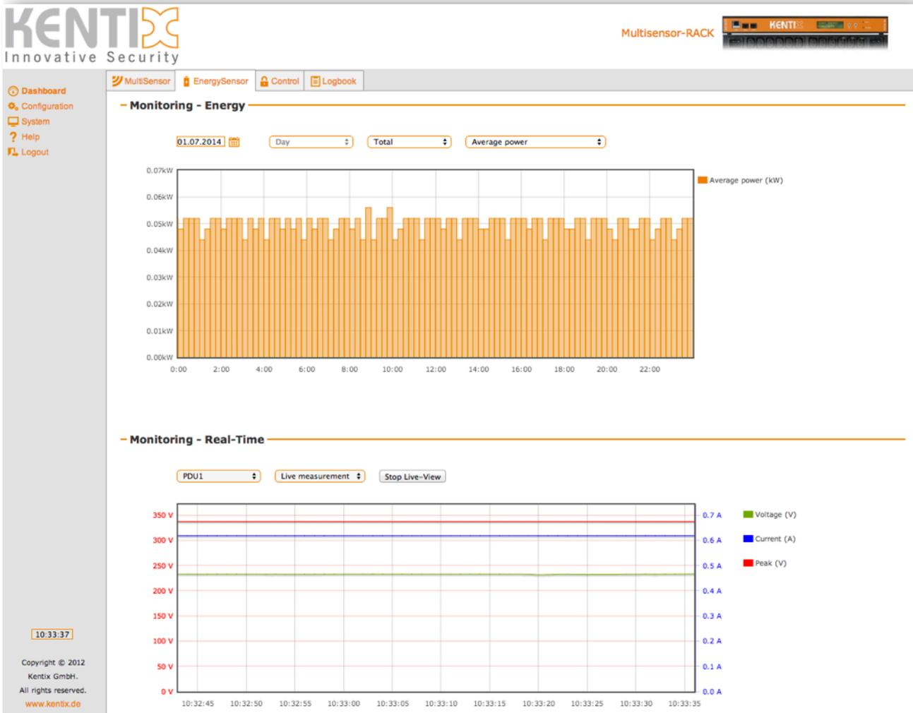
The real time graph shows the actual voltage profile, current and peak voltage for the last minute. Peak alarms will also be displayed. An occurring peak alarm will also be stored for later viewing.
