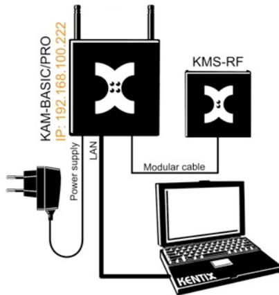
1. Connect AlarmManager and MultiSensor via Modular cable.
