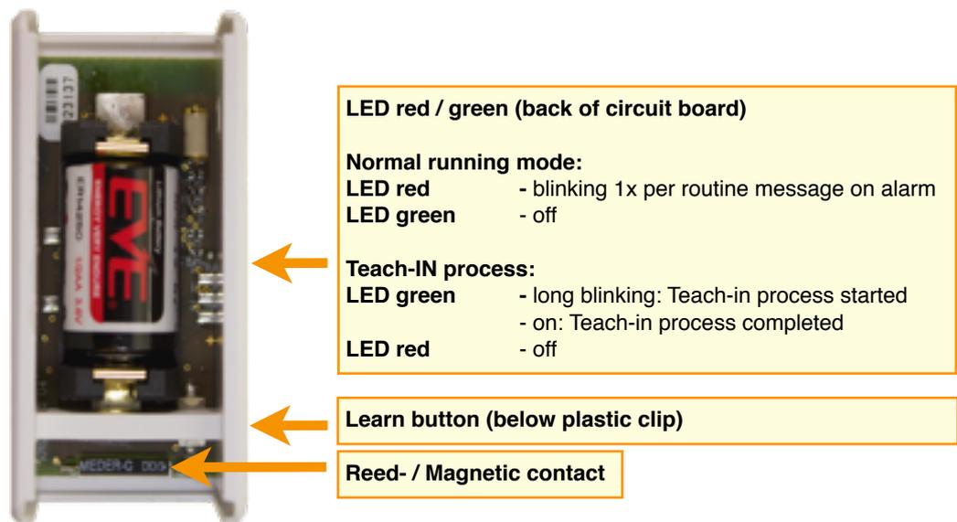
**Figure 2: MultiSensor-RACK-MINI**
