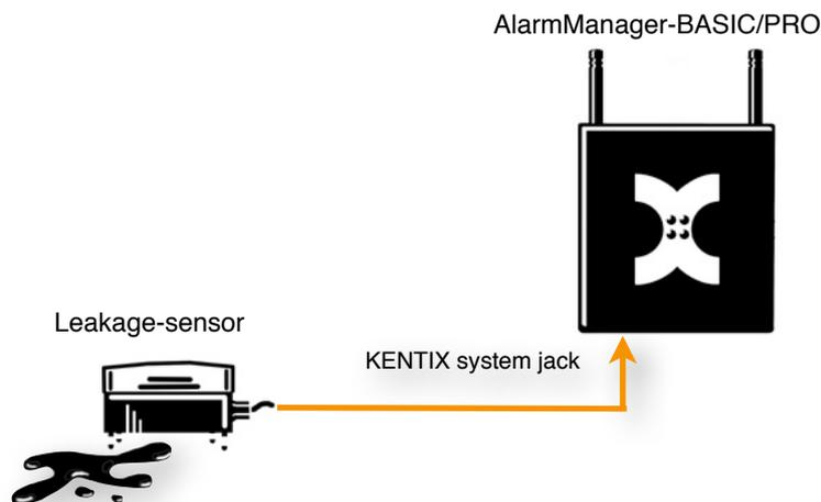
Plug the connection cable of the leakage-sensor into one of the System-jacks of the AlarmManager. The powering and alarming is done directly via the AlarmManager. With the ControlCenter enter a suitable name for the external alarm input and set the alarming of the input to „Always-Active“ for a permanent alarming. If the leakage sensor is working with opening the contact on an alarm, additionally change the alarm logic to „Open“.
