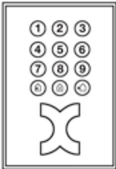
By pressing one of the keys "arming" or "disarming" followed by entering your personal code the zone assigned to the KeYPad is switched. Note that every user needs the according permissions to use a KeYPad.
