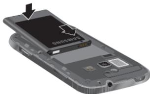
3. Replace the battery cover by aligning the cover and pressing it gently into place.
