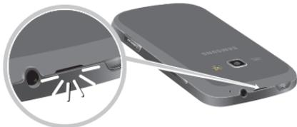
2. Insert the battery into the back of the phone, making sure to align the gold contacts.
