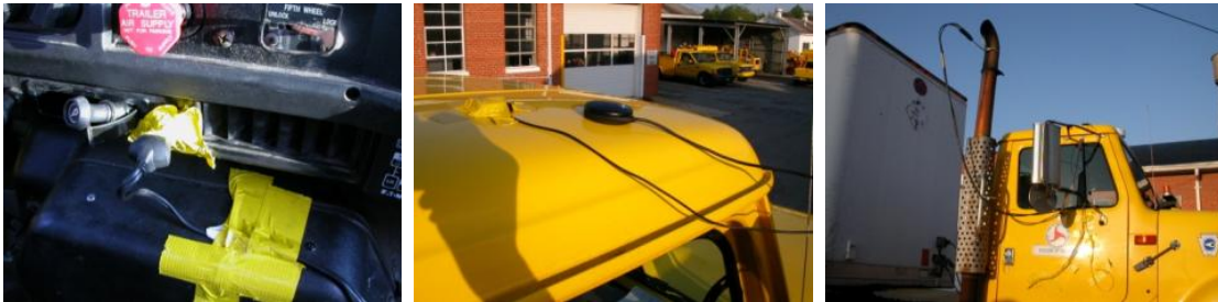
Figure 21. Installation of the Portable Emissions Measurement system (PEMS) Power Cable, GPS Receiver, and Exhaust Sampling Lines in a Truck 215-5715:
