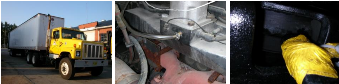
Figure 22. Installation of the Portable Emissions Measurement System (PEMS) Sampling Hoses and Engine Sensors in a Truck 215-5715:
