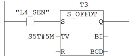
Networks 1 to 4 are used to program the life span of the signals from movement sensors. If a movement is detected, the timer output is activated. When the signal from the sensor disappears, the timer is started and the output is kept active during the time written in input TV. When a new signal is detected from the sensor, the timer is reset.
