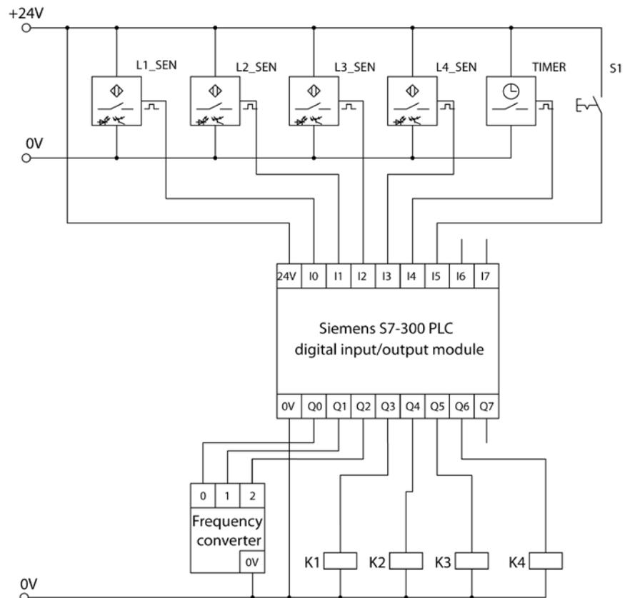
Fig. 0.3. Electric diagram for control circuit (low voltage part)
