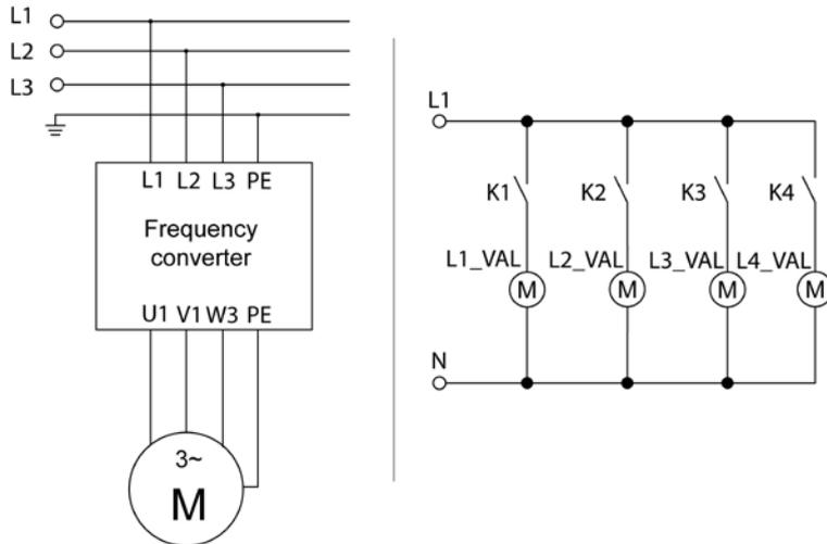
Fig. 0.2. Electric diagram for the power part
