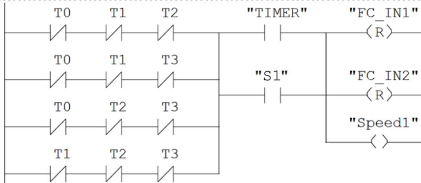
Network 6: *Ventilation works with higher speed*
