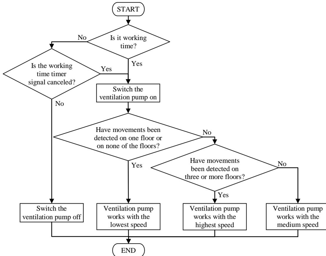
**Fig. 0.4. Flowchart of ventilation pump control**
