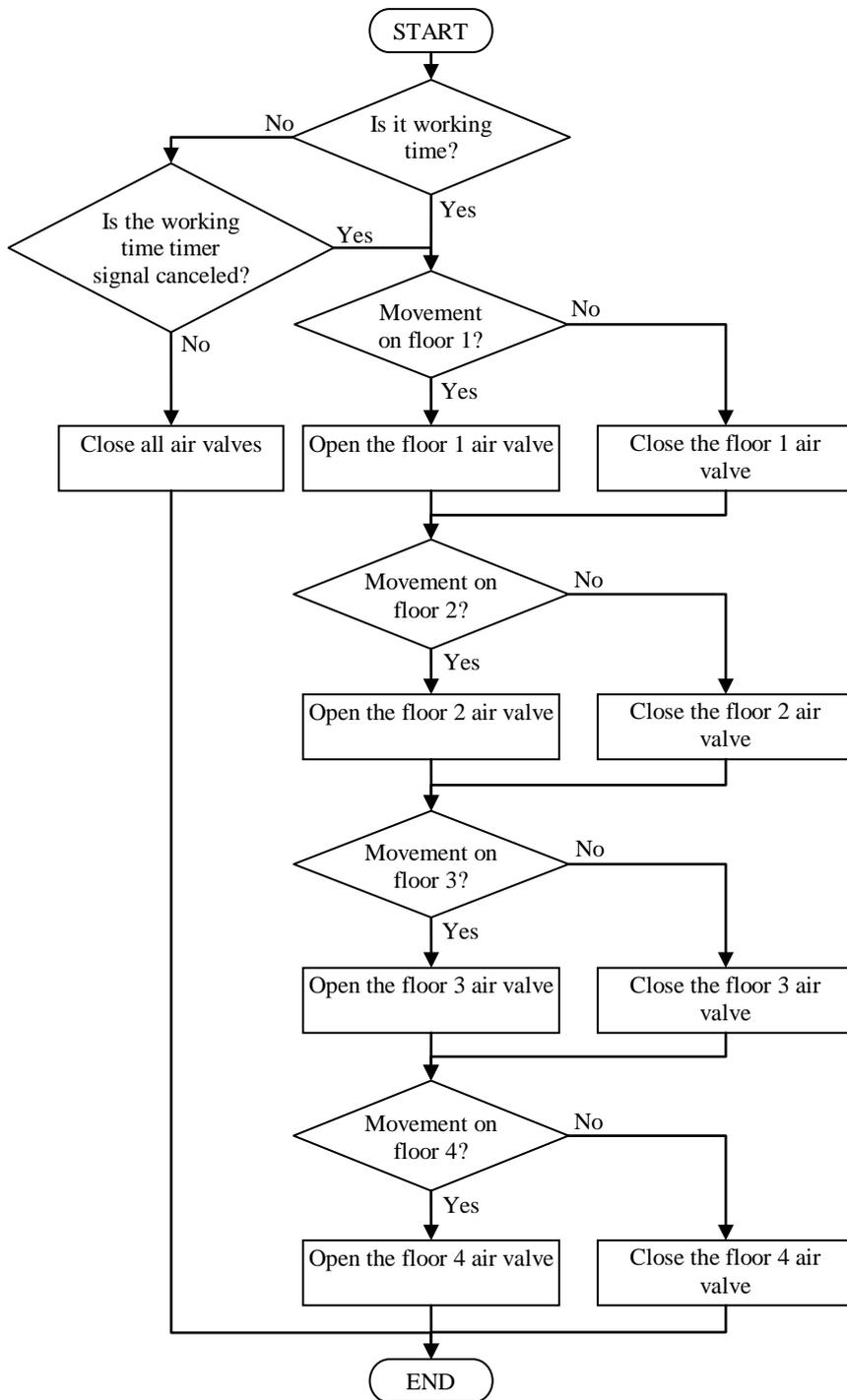
**Fig. 0.5. Flowchart of air valve control**
