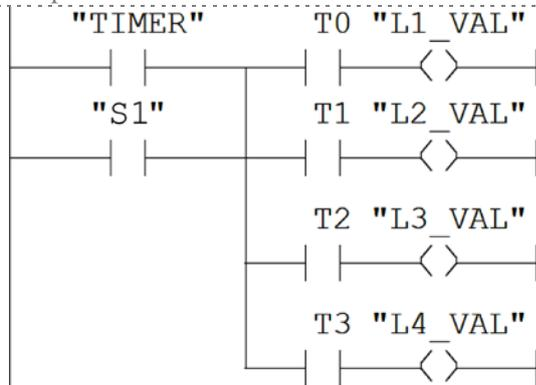
For example, when during work hours a movement is detected on floor 3, then this floor sensor signal is extended over 5 minutes (Network 3). The ventilation is set to work on the
