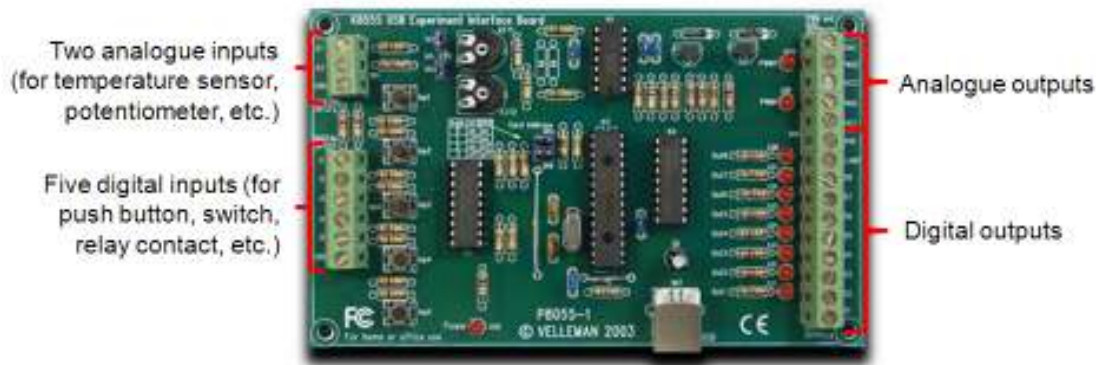
Figure 3 USB Interface Board (VM110) - Inputs and Outputs
