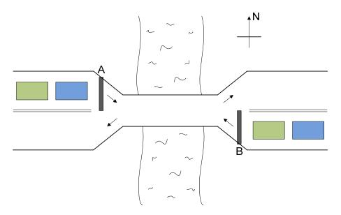
The bridge allows an East-West road to traverse a river, but is narrow and only allows traffic to cross in one direction at a time. To ensure adequate traffic flow, boom gates have been installed at either end of the bridge to ensure only one direction of traffic has access at any time.
