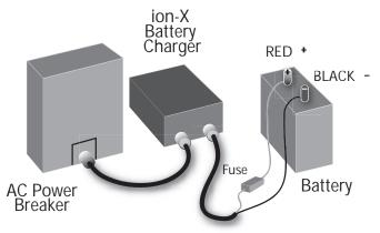
An inline fuse is provided on each positive (red) DC power cable, to protect the charger from inadvertent reversed polarity. In the event that your DC power cable fuse blows and requires replacement, refer to the General Specifications on Page 10 for the appropriate fuse rating to use with your ion-X Battery Charger.
