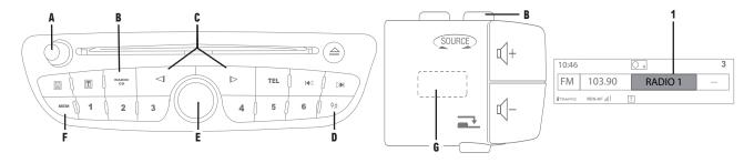
To switch the system on or off, press  ${\bf A}.$  Adjust the volume by turning button  ${\bf A}.$
