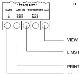
The list shows the y-axis values of the spectrum for the wavelengths marked during TRACK. The measured values will be ABS, %T, INTENSITY or 1D / 2D / 3D / 4D depending on the current mode.
