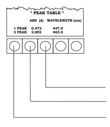
□ The list shows the positions and values of the peaks as calculated by the function selected in MANIPULATE PEAKS. The measured values will be ABS, %T, INTENSITY or 1D / 2D / 3D / 4D depending on the current mode and are sorted by wavelength. Each marker is identified as a peak, valley or zero crossing.
