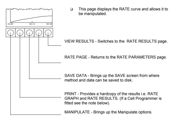
□ If more than one rate has been run in parallel using the Cell Programmer then three further print options are available: ALL OVERLAY, ALL SEQUENTIAL, and ONE RESULT.
