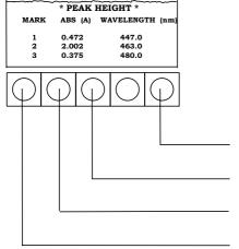
☐ This page shows the position and values of the wavelengths and the peak height as selected by the PEAK HEIGHT function.
