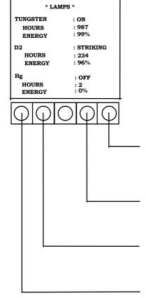
RESET HOURS – Displays a menu to choose whether the tungsten, deuterium or mercury lamp is to be reset. When selected resets hours and measures energy at the appropriate wavelength. ALLOW THE LAMP AT LEAST 10 MINUTES TO WARM UP BEFORE RESETTING ITS HOURS.
