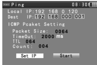
If IP camera or other ethernet equipment is not connected to the tester, “connect fail ” display on the screen. The sending and receiving packet amount is 0, the success rate is 0%. Press Enter
