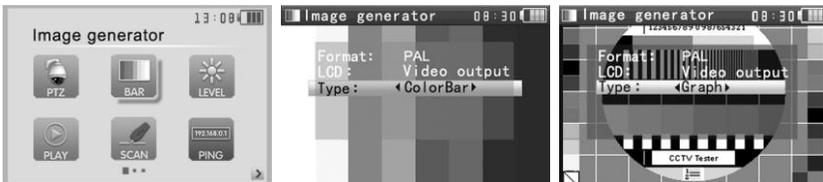
Test the Color- bar generator, support global PAL / NTSC standard color bar of different output formats
