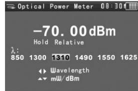
Data hold and Relative measuring use together, the data is yellow while the function is effect.
