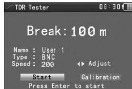
Press to “Adjust”, press **Enter/OPEN** to cable type, press to choose the cable style, press to “Speed” and press to adjust. While display length is the same as the actual length, press **Enter/OPEN** to save. It can be used for the same cable after the calibration.
