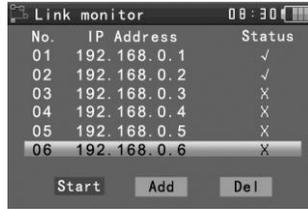
Add the IP address, make sure the network segment and the setting IP address are consistent, choose “start”, and press   to link monitor. If the status is “✓”, means the IP address is occupied, if the status is “X”, means the IP address is available
