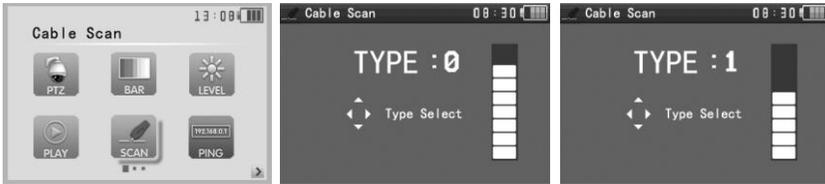
Turn on the cable scan; use the copper pin to search, the cable with loudest voice means it is connected with the tester. Four Audio types can choose. LED lamp is convenient to work in dark or at night. Press the button (+ -) to adjust the volume, use two batteries (size AAA)
