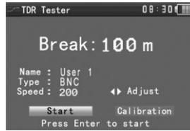
Built-in BNC, network cable, RVV control cable, Telephone line can test. 12 groups user-defined cable can be set.
