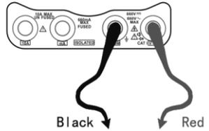
c. Before connect test leads across two sides of the capacitor under measurement, be sure that the capacitor has been discharged fully.
