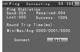
It’s normal that the first data packet will be lost when start the PING testing.
