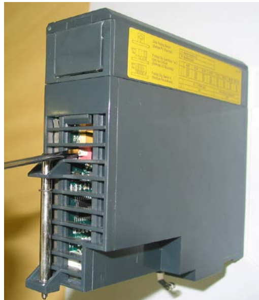
Figure 18. 10 – Locating the DF65 Rotary Switch
