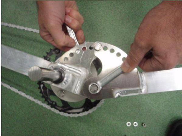
Connect the axis with the drive unit and fasten the bolts.
