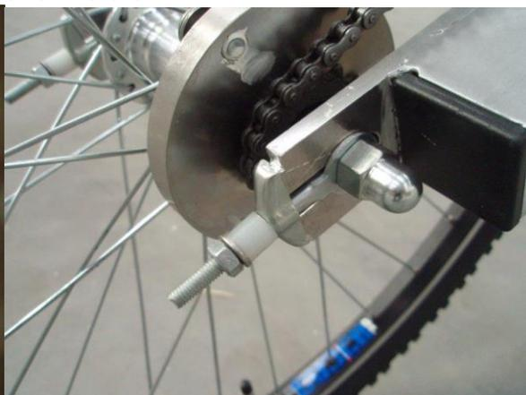
Adjustment of the chain gear
