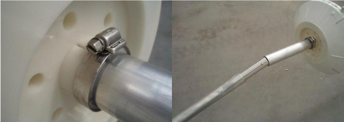
Mount the extension axis on the turn axis for 6 row operation.
