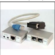
Bi-directional adapter to connect either an audio/composite video source (DVD player, satellite decoder, video recorder,...) or display (TV set, monitor, beamer,...) equipped with a SCART connector to a universal OmniMedia wall outlet through standard RJ45-RJ45 patch leads. Bi-directional IR-Bus interface for remote control transmitter or receiver wands. A unit can be used to bring AV signals to the ABI-EV1017S00 modulator or the ABI-EV1018S00 active AV splitter.
