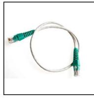
Characteristics: - RJ45 plug to RJ45 plug - Frequency range: 0 - 250 MHz Complies with: - ISO/IEC 60603-7 - ISO/IEC 11801 - ISO/IEC 15018 ABI-PC1001S45: 45cm - 0,026kg ABI-PC1001S60: 60cm - 0,032kg ABI-PC1001S75: 75cm - 0,036kg
