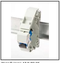
Fiberoptics multimode simplex SC feedthrough connector. The keystone latch mechanism maintains the SC connector coupler in the DIN-rail holder. Occupies 1 standard width on the DINrail. The device allows quick termination of Fiber access, backbone or FTTH links in a user premise, industrial site, automation equipment, etc.
