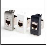
Wall outlet with 1 shielded RJ45 OmniMedia HD connector. Suitable for telephony, data and audio/video/TV applications. Fits in bTicino Axolute faceplates. The HD connector distinguishes from its predecessor by an unmatched EMC shielding efficiency throughout the UHF range, allows cable termination without dedicated tooling and the simplified colour coding reduces wiring errors.
