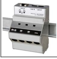
The ABI-ET2003S00 is a passive splitter module for the distribution of analogue (PSTN) phone and ADSL signals. An external ADSL filter is no longer needed thanks to the built-in filter. This simplifies the installation and comissioning of phone, fax and ADSL modem-router. The ABI-ET2003S00 does not provide the call-confidentiality function.
