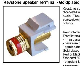
Keystone speaker terminal to terminate standard 1,5mm<sup>2</sup> to 6mm<sup>2</sup> speaker wire in wall outlet faceplates and patchpanels. Perfectly suited to prewire a home for stereo or surround multiroom audio. The strong gold plating guarantees long lasting corrosion free contact. Quick connection by screw-down or plug-in terminals. Front ring with a red or black band to identify the speaker wire polarity.
