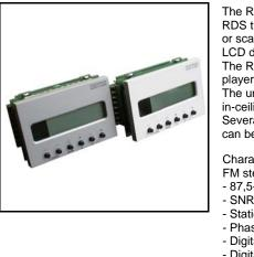
The Radio & Control Module fits in a double wall backbox. It incorporates a high-sensitivity FM RDS tuner with built-in clock radio and sleep function. The unit can be manually tuned into a station or scanned for the next station in the range. The name of the radio station is shown on the backlit LCD display.
