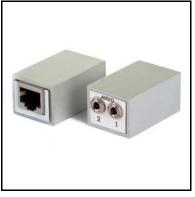
ABI-MM1009S00 is a miniature adapter that permits the transmission of two individual line level stereo signals over OmniMedia cable. The adapter is used for point-to-point or point-to-multipoint audio distribution in a Smart Media network. It can also be used as input coupler to connect a third party audio source to a multiroom multisource Smart Music network.
