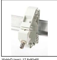
Fiberoptics multimode simplex ST feedthrough connector. The keystone latch mechanism maintains the ST connector coupler in the DIN-rail holder. Occupies 1 standard width on the DINrail. The device allows quick termination of Fiber access, backbone or FTTH links in a user premise, industrial site, automation equipment, etc.
