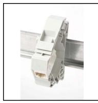
Unshielded RJ45-RJ45 feedthrough connector. The keystone latch mechanism maintains the connector in the DIN-rail holder. Adapted for telephony and data applications. Occupies 1 standard width on the DIN rail. Frequently used to bring ports of external devices (phone PABX, data switch,...) to the front panel of the Comm Center cabinet.
