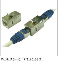
Shielded RJ45 jack to RJ45 jack coupler which allows quick interconnection of RJ45 patchcords to extend the reach of a temporary or semi-permanent connection. Standard keystone latch makes it compatible with a wide variety of faceplate brands and finishes (lists available on demand) or a keystone patchpanel like ABI-HE3002S24.
