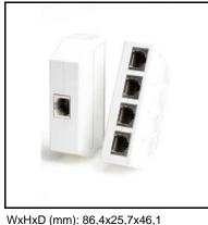
Splitter from one RJ45 jack to 4 RJ45 jacks. Each pair of the RJ45 jack is copied to pair 1 (pins 485) of the 4 RJ45 jacks. Can be used to connect four phones over a single cable link. Do not use for Ethernet, video or TV applications.
