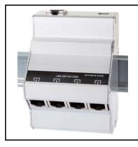
The IR-Bus HUB interconnects all IR-Bus transmitters and receivers linked through it's RJ45 ports on a common remote control bus. The hub is connected to a Smart Media power supply ABI-PS1001S11 and will power all connected IR-Bus transmitters and receiver devices via the cabling. This unit requires 5VDC from a power supply ABI-PS1001S11
