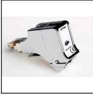
Video adapter to connect an analog camera or camcorder to a universal OmniMedia wall outlet by means of a standard video coax patch cable. Ensures impedance matching (100-75 Ohm). A pair can be used to set up a short RCA-RCA video extension, a single unit can be used to bring a video signal to the ABI-EV1017S00 modulator or the ABI-EV1018S00 active AV splitter.
