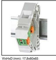
DIN-rail mounted speaker terminal to terminate standard speaker cable up to 2x2mm<sup>2</sup> in a DIN-rail cabinet. Perfectly suited to prewire a home for stereo or surround multiroom audio. The spring loaded contacts accept solid or stranded wires and retain good contact even in case of wire sagging.
