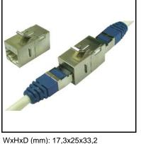
Shielded RJ45 jack to RJ45 jack coupler which allows quick interconnection of RJ45 patchcords to extend the reach of a temporary or semi-permanent connection. Standard keystone latch makes it compatible with a wide variety of faceplate brands and finishes
