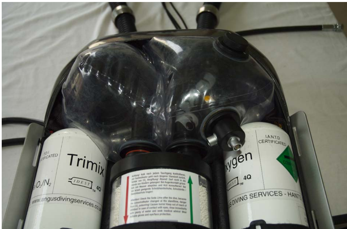
Positive Pressure Test (separate counterlungs shown)
