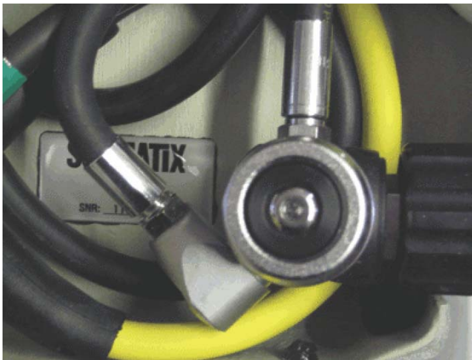
Oxygen 1 st Stage with the Interstage Pressure kit fitted to fix the IP at a predetermined level of 10bar (80m MOD) or 12bar (100m MOD)
