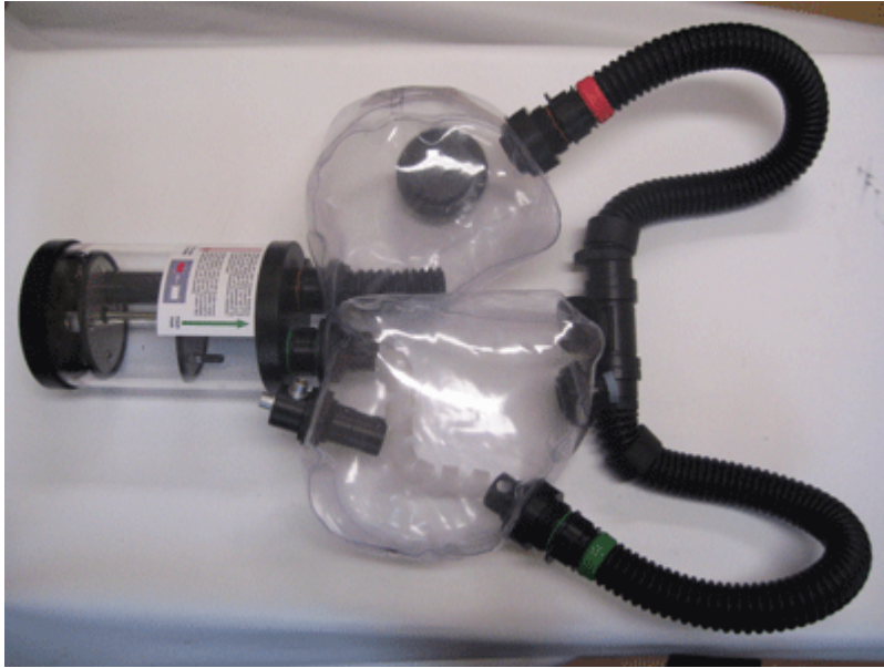
Breathing loop showing separate counter lungs
