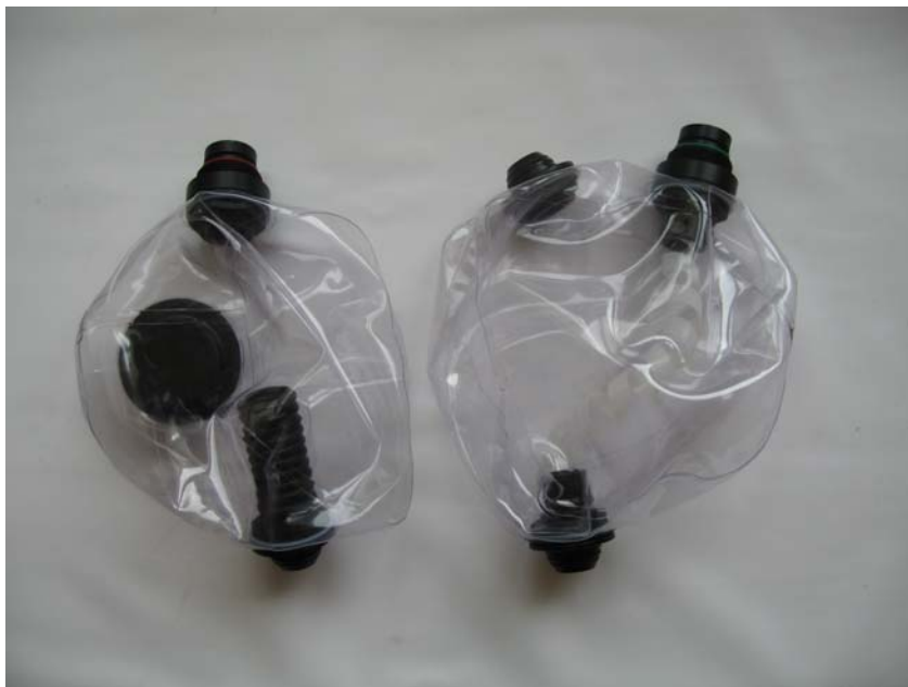
Separate counter lungs – Left: Exhale bag with over pressure valve and water trap. Right: inhale bag with 'anti-collapse' spiral inside
