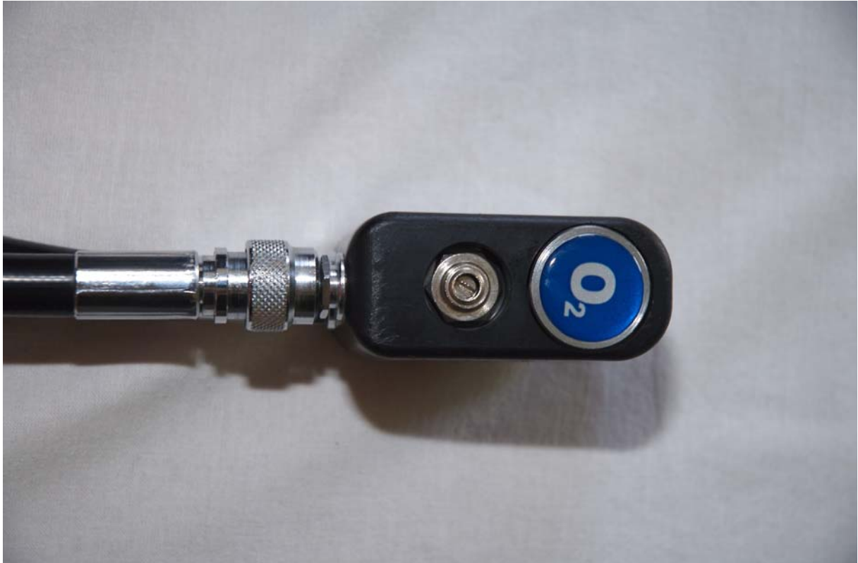
Pro Gas Booster manual oxygen addition unit showing needle valve and manual override button (in blue) and quick disconnect coupling
