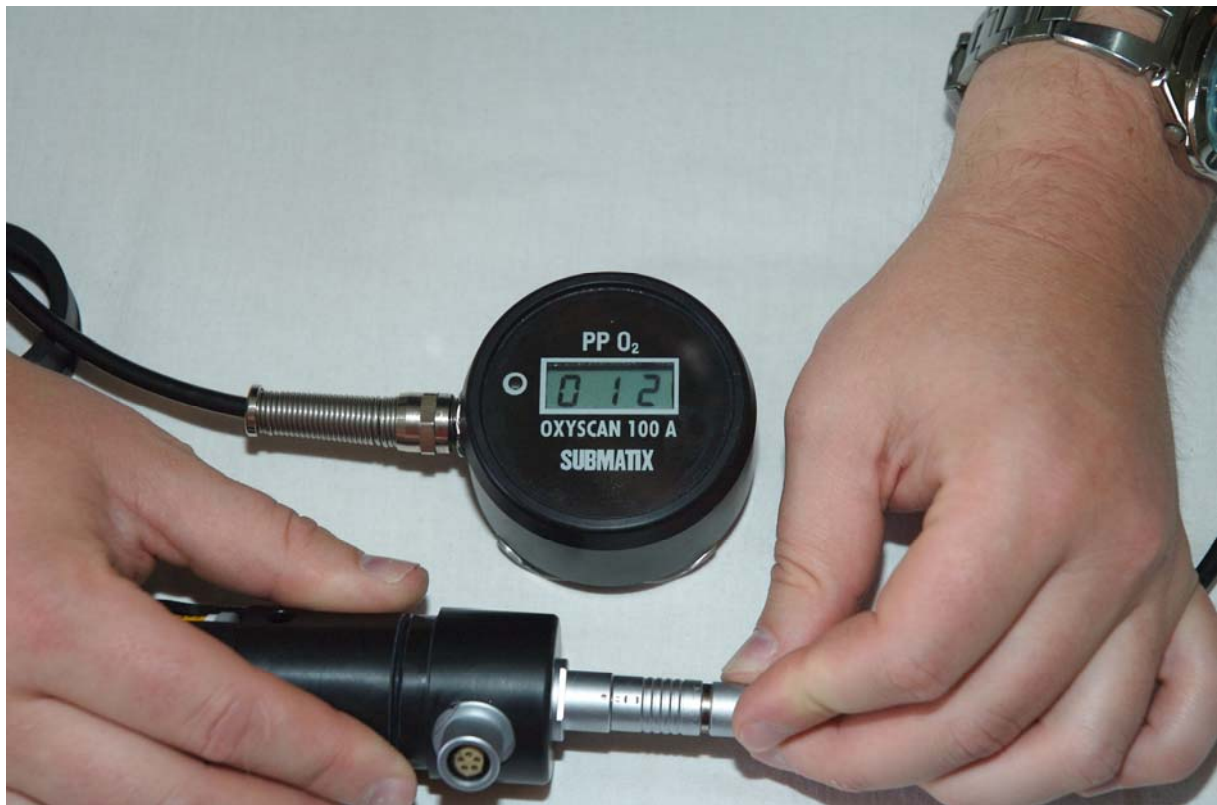
PPO 2 -monitoring system (Oxyscan)
