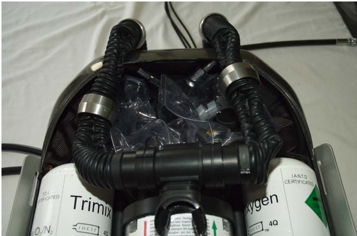
Negative Pressure test of the breathing loop (separate breathing bags)
