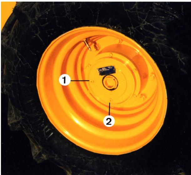
The wheel must be dismantled for checks and drainage. To do so, immobilise the machine and lift using a jack or a hoist.
