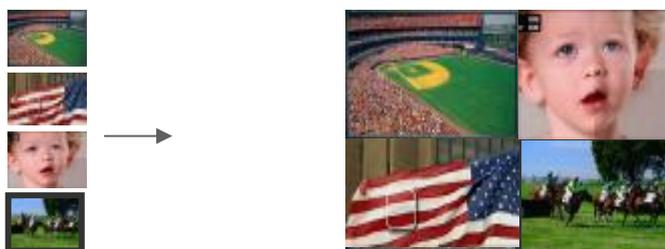
PBP mode: All signals can be any rectangular sharp display format at any size, without overlap between any windows.
