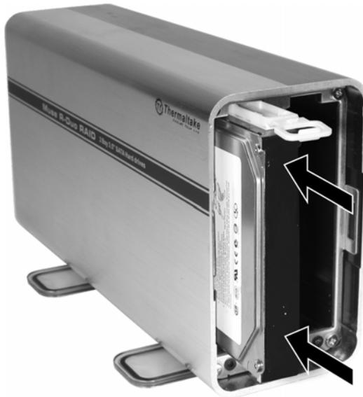
**NOTE:** Install the first hard disk drive on the left compartment, the second hard disk drive on the right compartment.
