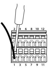
The terminal connections are numbered as follows:
