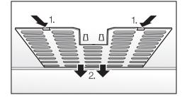
■ Unhook the filter cover ① in each side of the drawer and remove them along with the filters downwards starting from ②.
