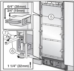
The installation aids (5) have been designed for the following total thicknesses of custom doors:
