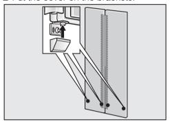
The number of lower brackets will depend on the width and the design of the custom door.
