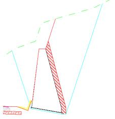
Composite Breast Wall: Composite Breast wall is similar to composite retaining wall. Some more parameters are added for breast wall portion. You can define a filter media layer in the outside breast wall portion.
