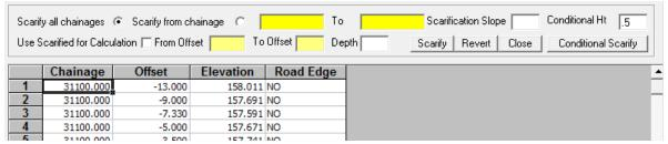
Now a new feature has been added in Scarification screen: *Conditional scarification* which takes into account the height difference criteria automatically and scarifies only those chainages which meet this criterion.
