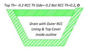
Separate Inner RCC Internal wall slope: In case your RCC lining has different slope for the internal wall, it can be easily defined with the new option. You can enter the slope to follow for right and left side for internal wall.
