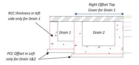
Separate Thickness of Inner RCC lining: You can specify the left and right RCC thickness of inner lining separately by separating both left thickness & right thickness with a comma e.g. 0.2, 0 means 0.2 thickness in left side and 0 offset in right side.
