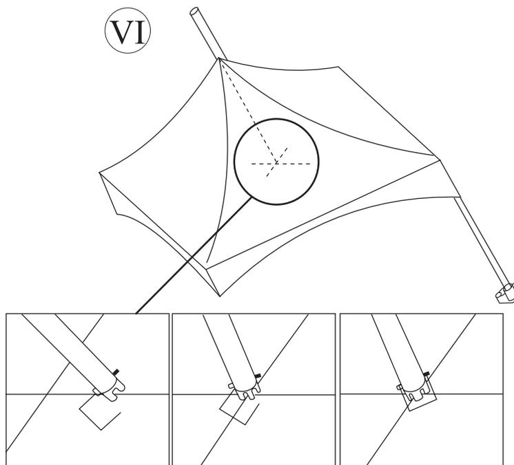
**11)** Install the remaining two legs (8') as done in step #9 be sure the smaller holes of the base plate is facing the interior of the tent.
