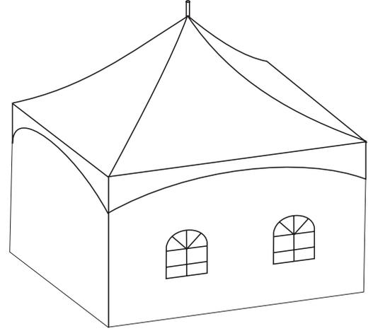
**13)** Your tent should be erected. Now adjust the ratchet rope locks to properly tension the tent top. Adjust all four corners until the tent top is tight (See Diagram: IX).
