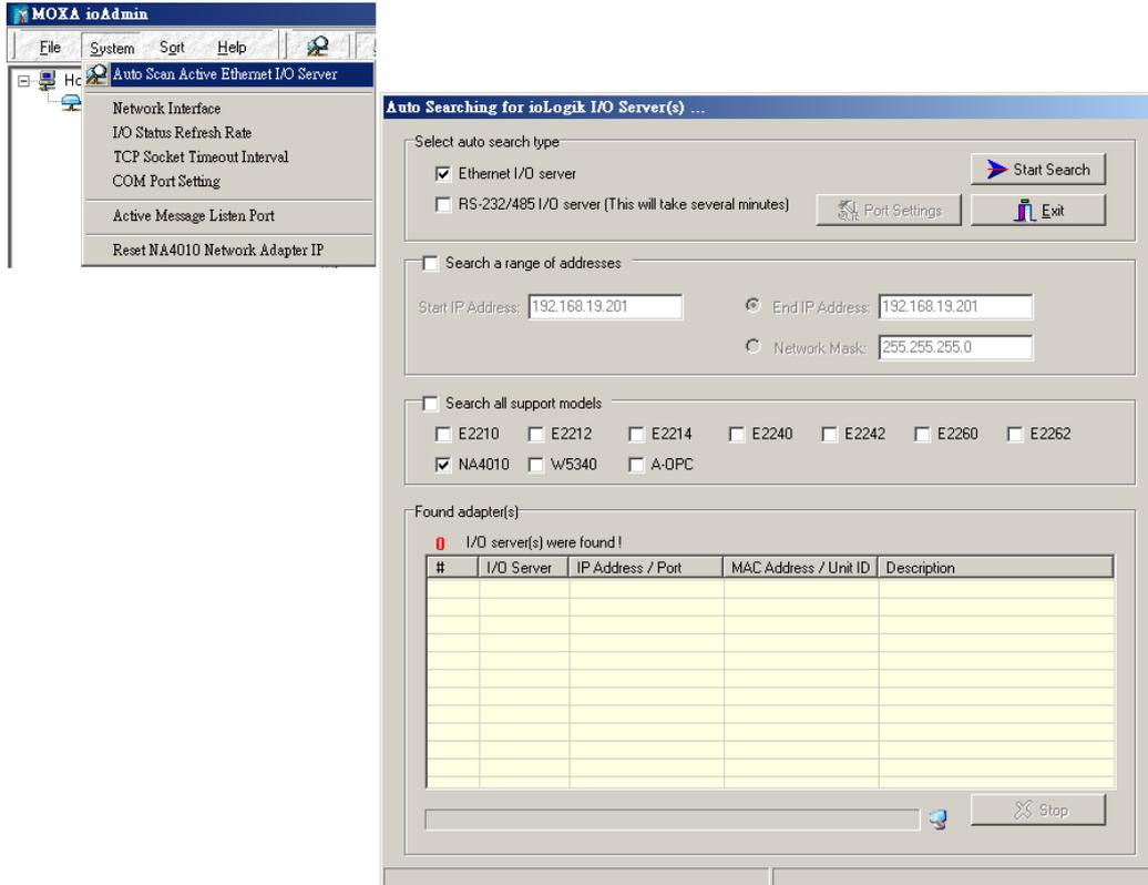
Select **Ethernet adapter**, and then click on **Start Search**. ioAdmin will start searching for installed NA-4010's on the network.
