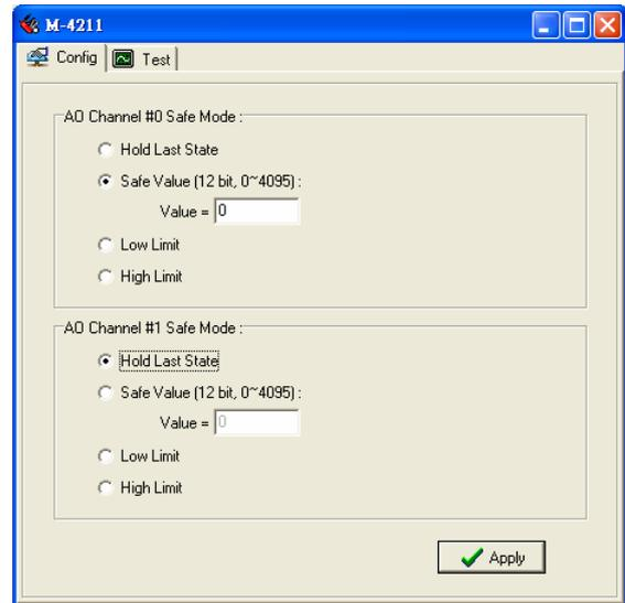
You may test if the analog output channel really works over the network. Click on the "Test" tab on the "Config" page. Scroll the output level, and then press "Test." At this point, you can change the level of the analog output point.
