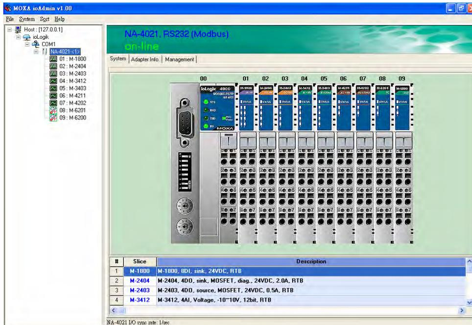
The left frame of ioAdmin shows all I/O Servers found on the network. The upper right frame indicates the combination of all I/O modules by slot number. The lower right frame lists detailed information for installed I/O modules.
