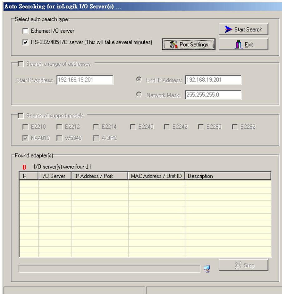
Click **Port Settings** to configure the COM port and baud rate, data bit stop bit, and parity for further communication. Click **Start Search** to search for connected RS-485 or R-232 I/O Servers.
