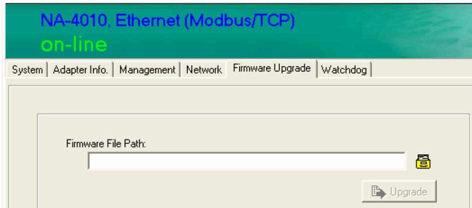
Click on the file icon and select the firmware. Press **Upgrade** when you're ready. During the firmware upgrade, DO NOT turn the ioLogik 4000's power off.
