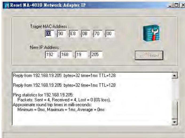
ioAdmin automatically changes the IP address and tests the new IP.
