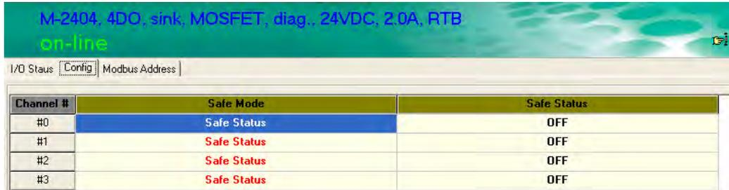
To check the Modbus Address, click on the "Modbus Address" tab.
