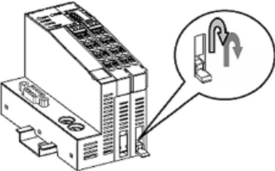
**Step 2:** Pull out the I/O module.
