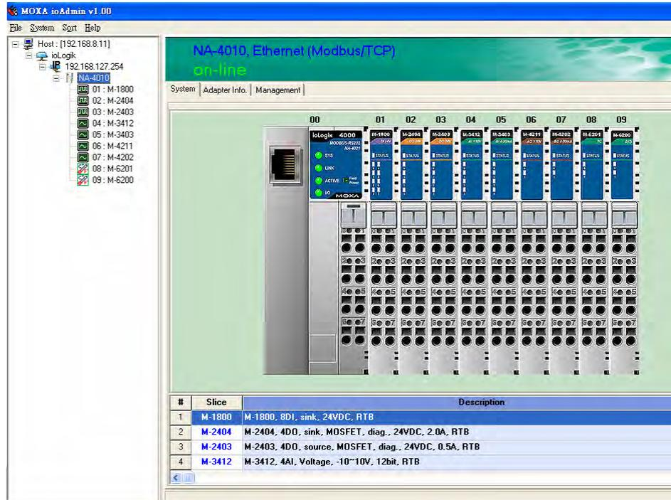
The left frame of ioAdmin shows the I/O Servers connected to the network that were located by the search process. The upper right frame indicates the combination of all I/O modules by slot number. The lower right frame lists detailed information for installed I/O modules.
