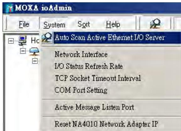
ioAdmin can automatically allocate available COM ports on the host computer and scan Unit IDs from 01 to 99 for each COM port. However, it takes longer to finish the process. A more efficient and faster method is to select **Only Search: COMx** and search designated COM ports. Note that ioAdmin supports Modbus/RTU. In a Modbus/ASCII environment, configure the Network Adapter using Modbus/RTU, and then switch back to Modbus/ASCII for field operation.
