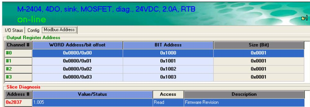
There are three columns for Modbus Address. According to the Modbus standard, there are two methods to access I/O channel. One is access by Register, and the other is by Coil. Each I/O channel can be accessed via the Register or Coil method.
