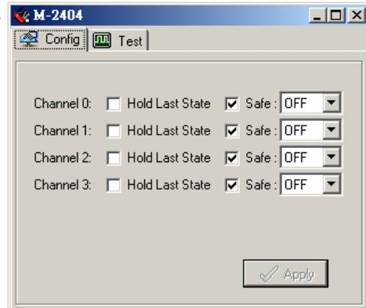
You can test to make sure the digital output channel works over the network. Click on the "Test" tab in the "Config" page. Press the switch, and then press "Test." At this point, you can change the status of the digital output point.
