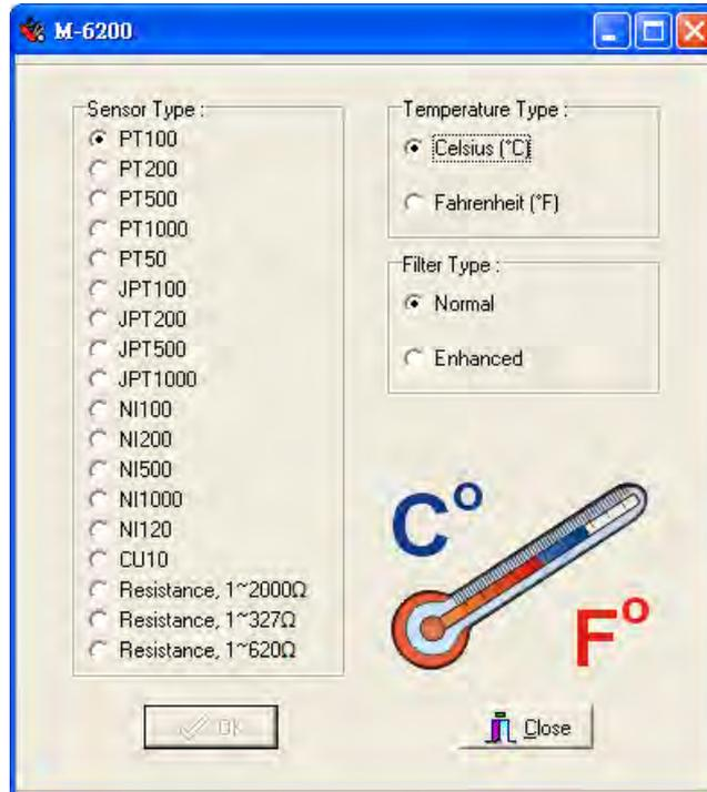
On this page, you may set up the sensor types and temperature unit. Note that the configuration applies to all channels in the same module. The related model is M-6200. The **FilterType** represents different sampling times. In Normal mode, the conversion time is about 200 msec. In Enhanced mode, the conversion time will be about double, or around 400 msec.
