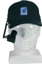
Fig 3: Display mounted below your eye
