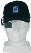
Fig 1: Display mounted above your eye
