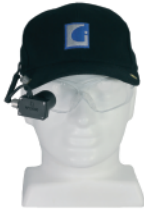
Fig 2: Display mounted at side of your eye
