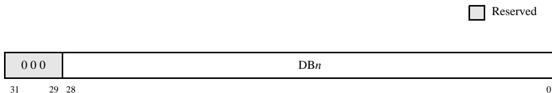
Figure 9-3. Outbound Doorbell Register (ODBR)
