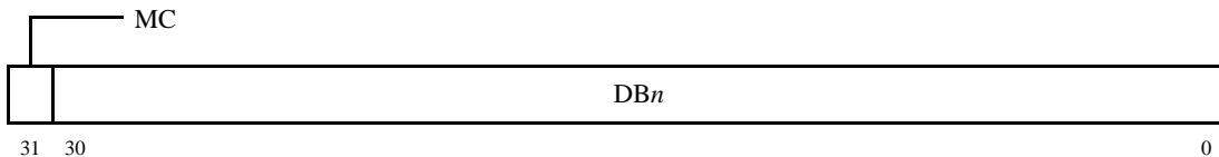
Figure 9-2. Inbound Doorbell Register (IDBR)
