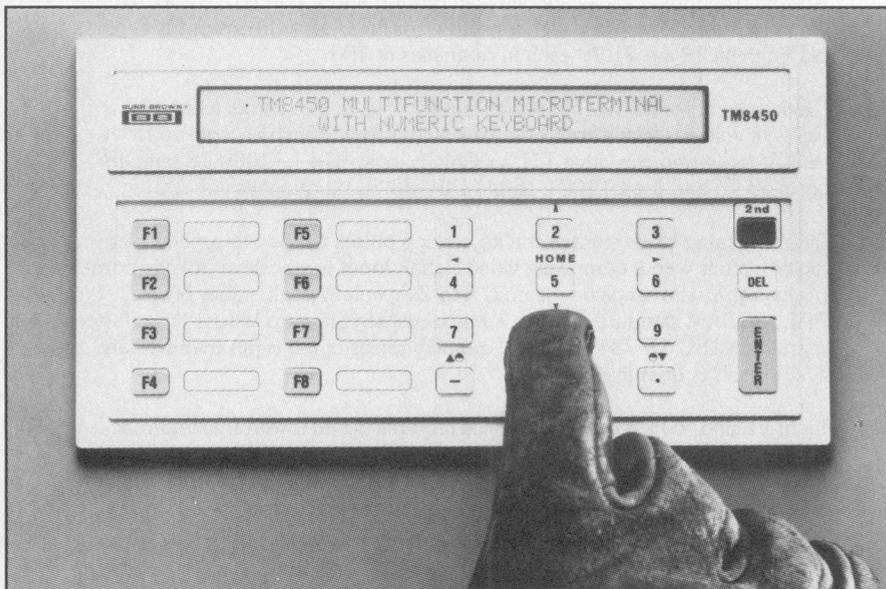
The base unit of Burr-Brown's TM8450 features a backlit LCD and a 23-key numeric keyboard. Eight keys can be programmed for 16 separate functions.
