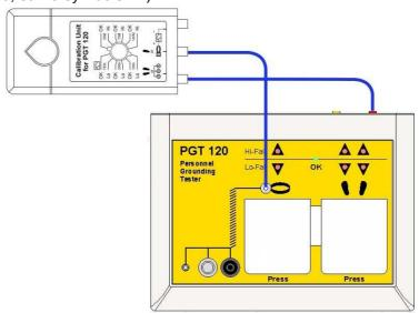
Set the marked lever of the rotary switch in succession to the positions mentioned below. Press the <u>right</u> contact electrode for each measurement.
