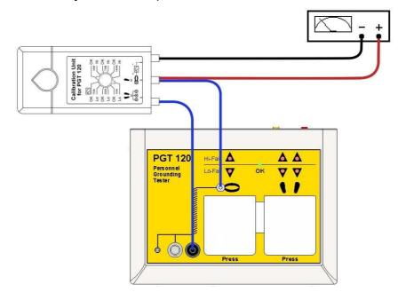
Use a DC-voltmeter with impedance Ri  $\geq$  10M $\Omega$ , preferably measuring range 2V.
