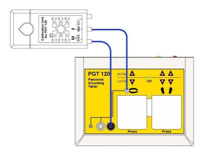
Set the marked lever of the rotary switch in succession to the positions mentioned below. Press the <u>left</u> contact electrode for each measurement.
