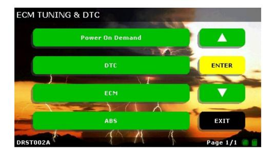
The DTC option is for checking *Diagnostic Trouble Codes*. Typically a check engine light will be present when there are codes to check for. The Smarty will provide a readout of what the code is.
