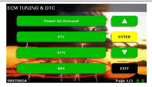
The ABS option is for tire size adjustments. This will allow you to correct the speedometer when running an after-market tire size. If you spend most of your time towing or loaded, we recommend loading the truck before taking your measurement (for best results). Note this option will not be present until the truck is programmed with a CaTCHER software.
