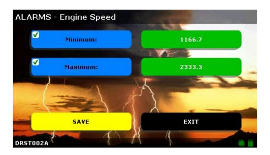
The menu here is fairly simple: A minimum and a maximum alarm. Check a box for each alarm you would like to use, and adjust the value by pressing on the green box to the right. You will see a keypad identical to the previous ones.
