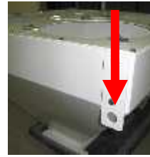
Lifting hook in SHIPPING position
