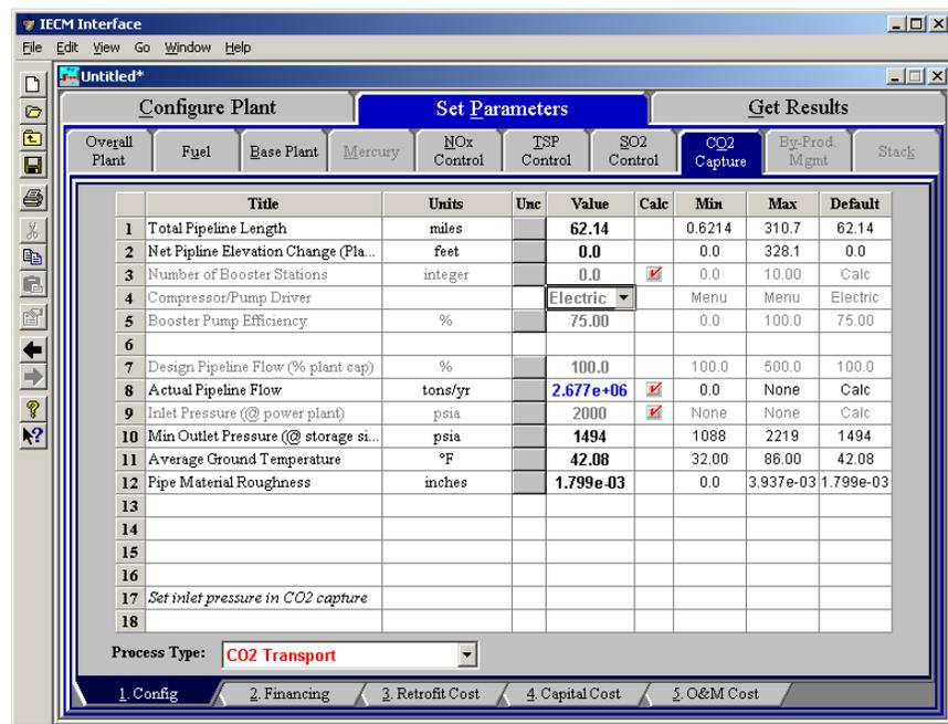
CO<sub>2</sub> Transport System – Config. input screen.
