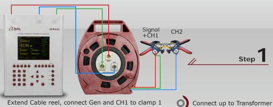
Extend Cable reel, connect Gen and CH1 to clamp 1 and CH2 to clamp 2. Connect clamps together and check for 0dB throughout the sweep range
