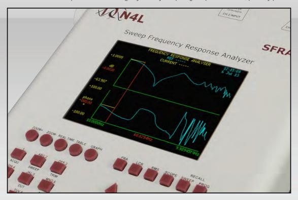
The picture above illustrates the ability to compare plots during a sweep, the reference plot is shown in blue and recalled from internal memory. This enables the engineer to detect immediately any difference between the plots giving the engineer the option to cancel the test.
