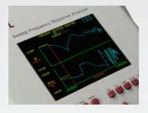
Set up the sweep and enter transformer parameters in the DUT menu, save sweep to the SFRA45's 1GB internal memory (Data can be saved in XML format and imported to SFRAComm later)
