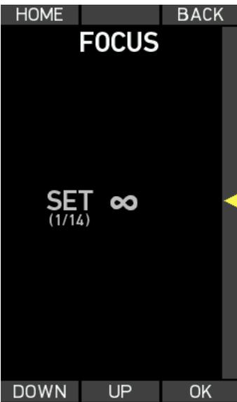
Use the focus knob to drive the lens focus scale to its infinity mark.
