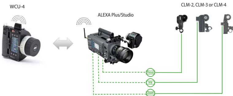
Fig. 1: WCU-4 controlling three motors on ALEXA Plus
