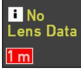
Pre-marked focus ring active, but no lens data available from motor controller.
