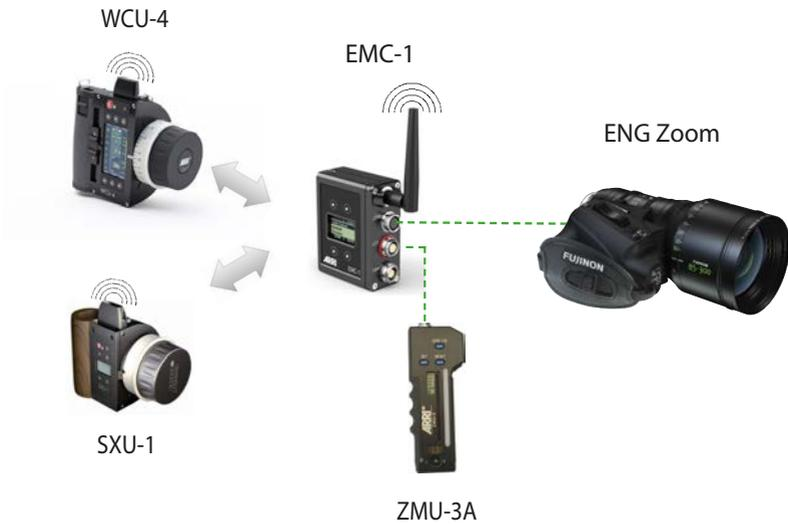
Fig. 7: Sample network setup with EMC-1
