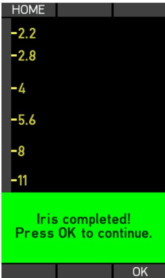
After entering all iris points, press the OK soft button to return to the *Select Axis* screen.
