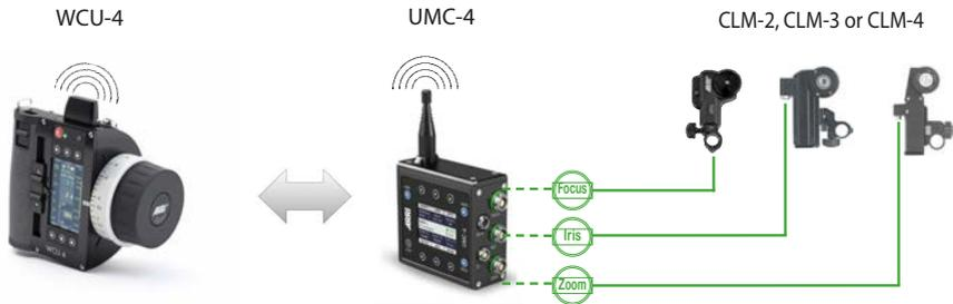
*Fig. 2: WCU-4 controlling three motors on UMC-4*
