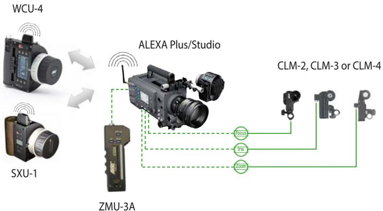
Fig. 5: Sample network setup with ALEXA Plus
