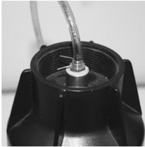
Push tube onto barbed fitting all the way, until it is against the base of the fitting. Then use pliers to slide tubing clamp down tubing to below the barb.
