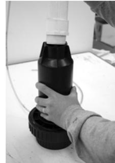
Finally, with the tubing securely fastened to the pressure bell and all the tubing fed through the pipe, thread the adaptor to the top of the pressure bell (Hand Tighten Only!).
