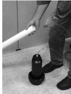
With the tubing securely attached to the pressure bell, feed it through the PVC pipe from the side with the male adaptor already attached.
