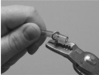
Use pliers to slide tubing clamp onto end of the tubing approximately 1 inch.
