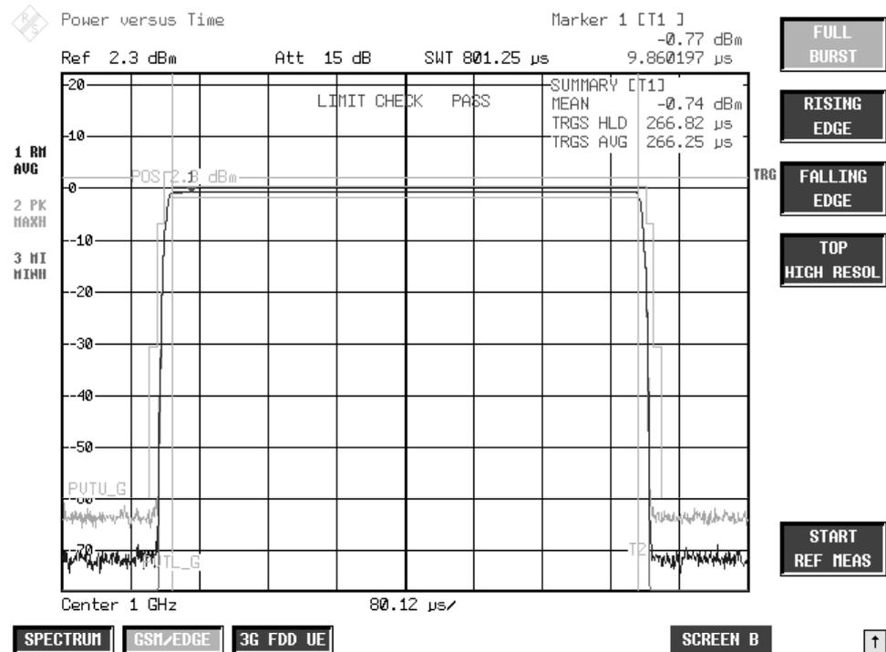
Figure 2-7 PVT single slot measurement – FULL BURST
