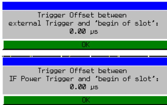
**Note:** The values determined here for the GSM trigger offset must be specified in remote-control mode for correct synchronization with the `TRIGGER[:SEQUENCE]:SYNChronize:ADJust:EXTernal`, `TRIGGER[:SEQUENCE]:SYNChronize:ADJust:IFPower` or `TRIGGER[:SEQUENCE]:SYNChronize:ADJust RFPower` commands. IEC/IEEE bus command-- (the GSM trigger offset must be specified in remote-control mode)
