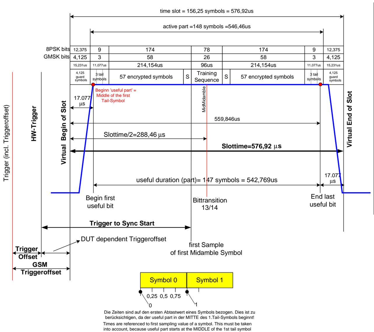
Figure 1-4 Trigger and time references
