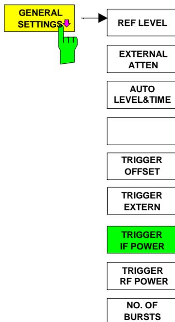
Pressing the *GENERAL SETTINGS* softkey opens a submenu for setting the major parameters of the GSM/EDGE base and mobile station tests application.
