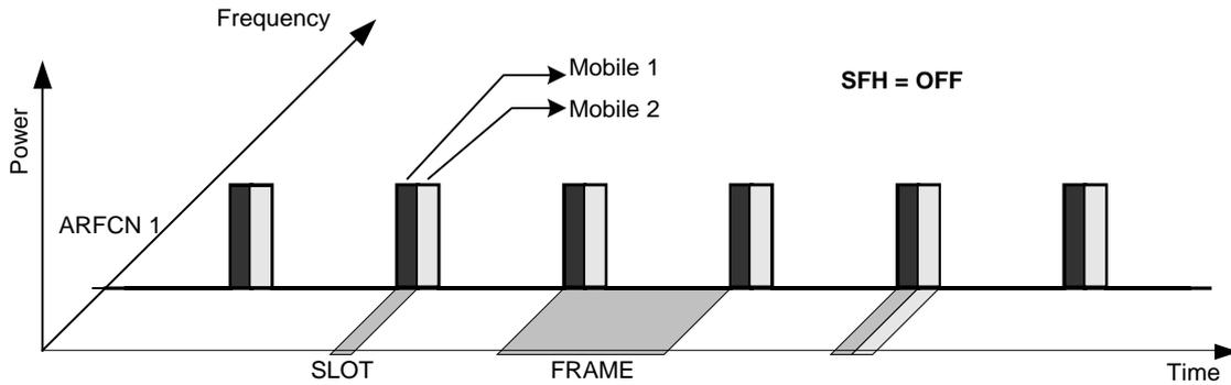
**Mobile 1 transmitting on same frequency, mobile 2 transmitting on different frequencies**
