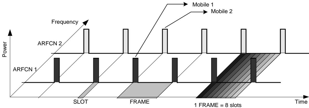
**Mobiles transmitting on the same frequency at different times: TDMA**
