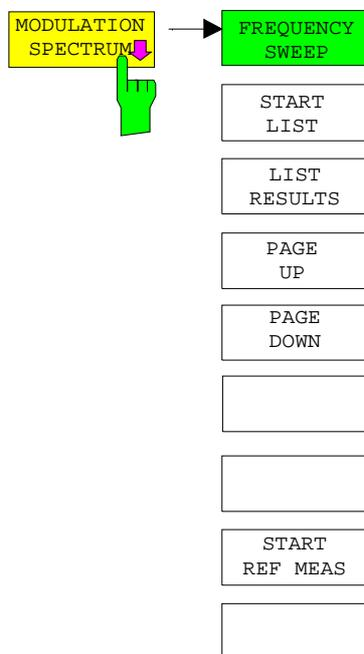
The *MODULATION SPECTRUM* softkey calls the submenu for measuring the spectrum due to modulation. In the default setting, the spectrum analyzer measures the spectrum due to modulation in the frequency domain (*FREQUENCY SWEEP*).
