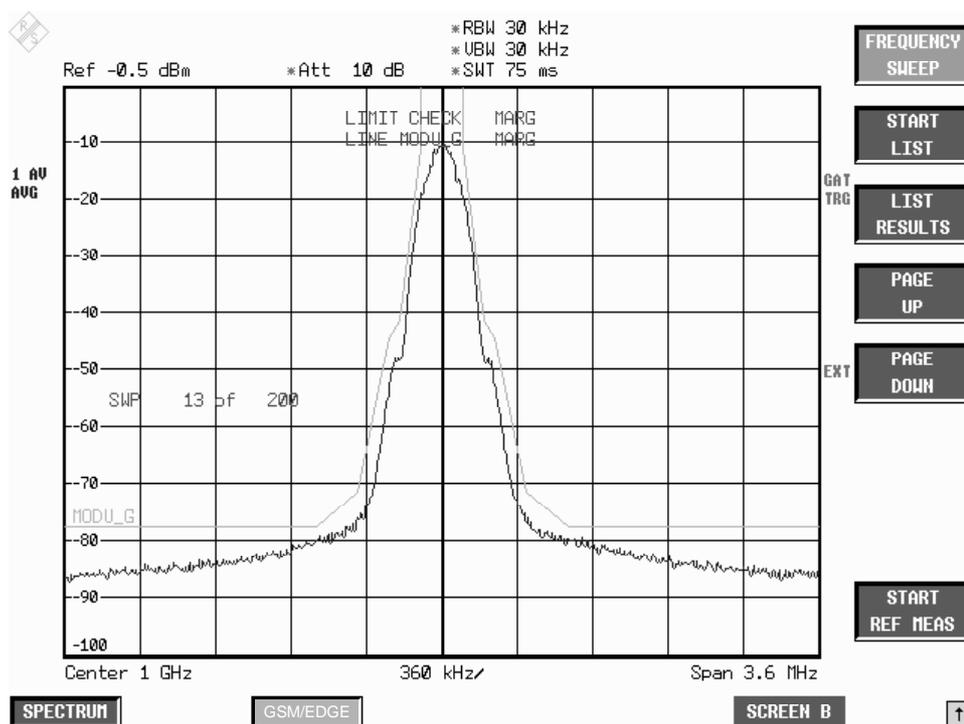
Figure 2-12 Spectrum due to modulation in frequency domain
