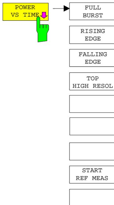
Press the *POWER VS TIME* softkey to start measurement of carrier power versus time and open a submenu for configuring the display. The power of the burst is also measured as centered relative to the midamble and displayed.
