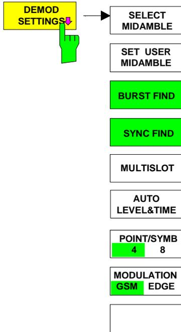
Pressing the *DEMODO SETTINGS* softkey opens a submenu for setting the major parameters of the demodulator in the GSM/EDGE application.
