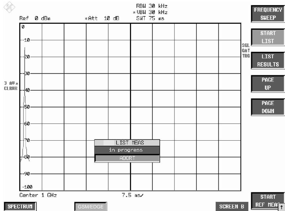
Figure 2-13 Time domain measurement in progress
