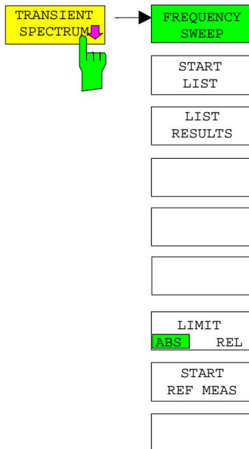
Press the *TRANSIENT SPECTRUM* softkey to call the submenu for measuring the spectrum due to transients. In the default setting, the SPECTRUM ANALYZER measures the spectrum due to transients in the frequency domain (*FREQUENCY SWEEP*).
