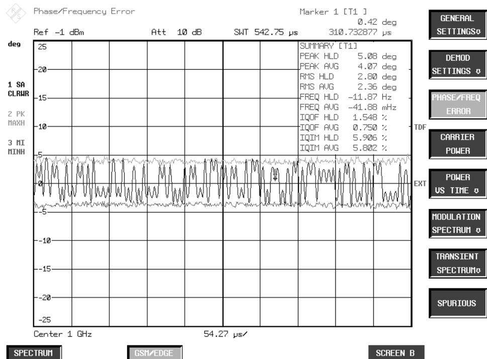
Figure 2-5 Measurement of phase and frequency error
