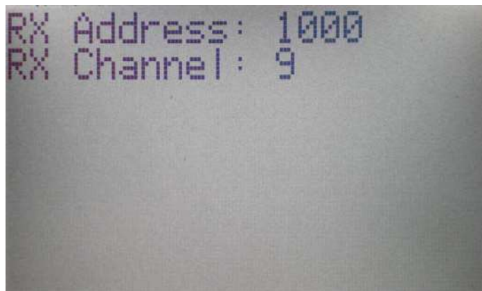
Figure 18: MHR Access Code and Channel
