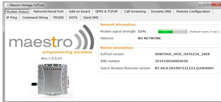
After connection check you will first arrive on this Modem Status tab. It displays the reception signal strength (refreshed every 5sec.), your SIM card network name. And all the versions of the embedded application. Useful to send a screen shot of this tab to your distributor, or Maestro contact, when you encounter any problem with your modems.
