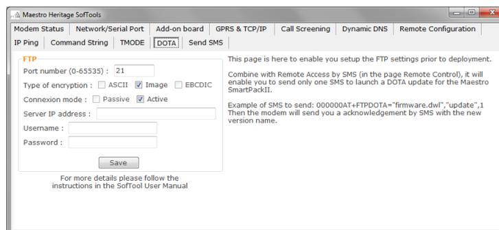
This tab allow you to first setup your FTP server for DOTA upgrade, then combine with remote access, this will allow you to update your modem firmware with only one SMS !
