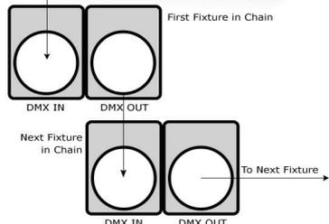
**Step 3:** Connect other fixtures in the chain from output to input as above. Place a DMX terminator on the output of the final fixture to ensure best communication.
