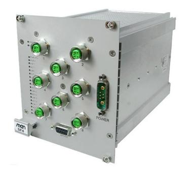
The SF4 is a stand-alone, unmanaged industrial Fast Ethernet switch that comes in a compact 3U, 22HP, 19" cassette. It provides eight channels at the front panel accessible through M12 connectors.
