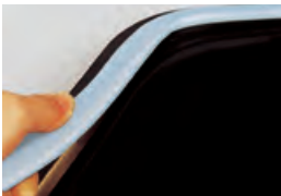
Channel Installation 1. Apply an adhesive silicone between the channel base on fixture housing to prevent slippage and stretching over time. 2. Press LED Neon-Flex™ RGB into the channel with even pressure from the beginning to the end.
