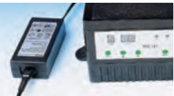
Low Voltage Power Supply and Controller 1. SRC-181 Controller 2. Switch Power Supply
