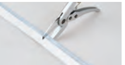
Cutting Mark LN-FX Must be cut only on the indicated mark
