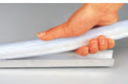
Linear Installation 1. Aluminum Channel LN-FX-RBG-CH 2. Apply an adhesive silicone between the channel base on fixture housing to prevent slippage and stretching over time
