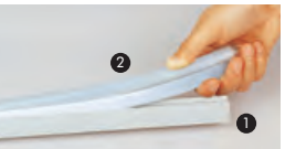
Linear Installation 1. Aluminum Channel LN-FX-CH 2. Apply an adhesive silicone between the channel base on fixture housing to prevent slippage and stretching over time
