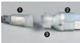
Front connector includes 1. Electrical plug 2. Male connector (with waterproof rubber ring) 3. M24 screws
