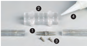
Splicing Connector 1. 2-Way Double Pin Splicing Connector 2. Plastic Shell (2 Piece) 3. Self-tapping Screws 4. Silicone Adhesive
