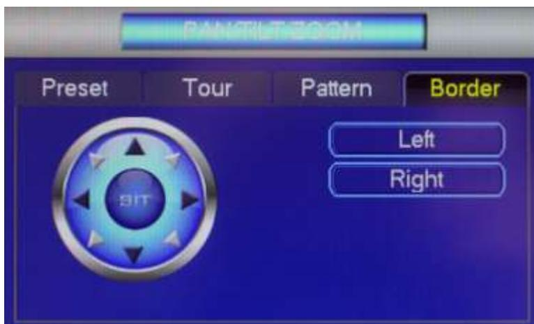
For border settings, the direction buttons can be used. Use the left/right buttons to set the borders.
