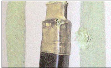
Damaged webbing and shock absorber protector
