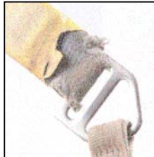
Wear at the end of the absorber loop at connection
