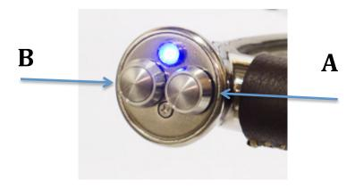
When stopping the caddy a "parking brake" automatically engages. The LED will flicker 2 Quick and 1 Slow, indicating "brake" is set. To release the parking brake, press and hold the B button for one second till LED is solid blue. When trolley is
