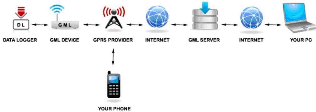
From your PC, you can not only download the SD1 data (which has been uploaded by the GML1 device) but with an SD1 you can also check on the operation, status and battery life of the SD1. This is discussed in full detail further on in this manual.
