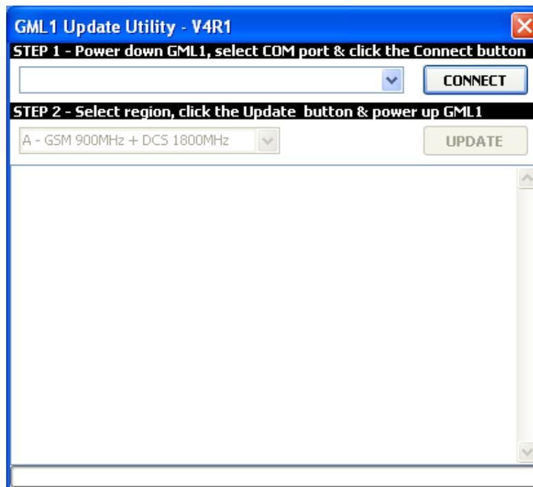
To program the firmware in the modem connect the GML1 unit to a spare serial port on your computer (you may use a USB to RS232 converter cable). After you run the V4R1 program and select the COM port from the drop down list please make sure that GML1 is powered down before clicking on the CONNECT button. In the example below COM1 port has been selected as the serial port connected to the GML1 unit.
