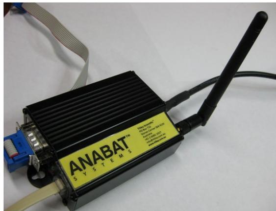
The SD1 connects to the GML1 RS232 port via a DB9 male to DB9 female straight through cable. Please note that a shielded type cable is recommended and the cable should not be longer than 15 meters (even less for low quality cables). A feature of the GML1 is that it can share a power supply with the SD1. Furthermore, it connects to the Internet only when the data has to be uploaded from the SD1, thus ensuring minimal power drain.
