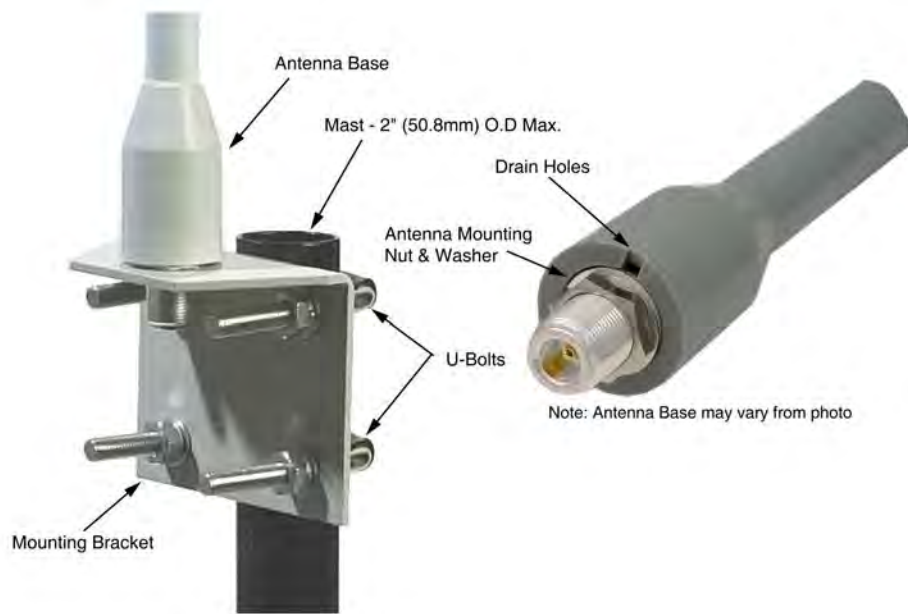
Figure 4-4 Omnidirection antenna mounting
