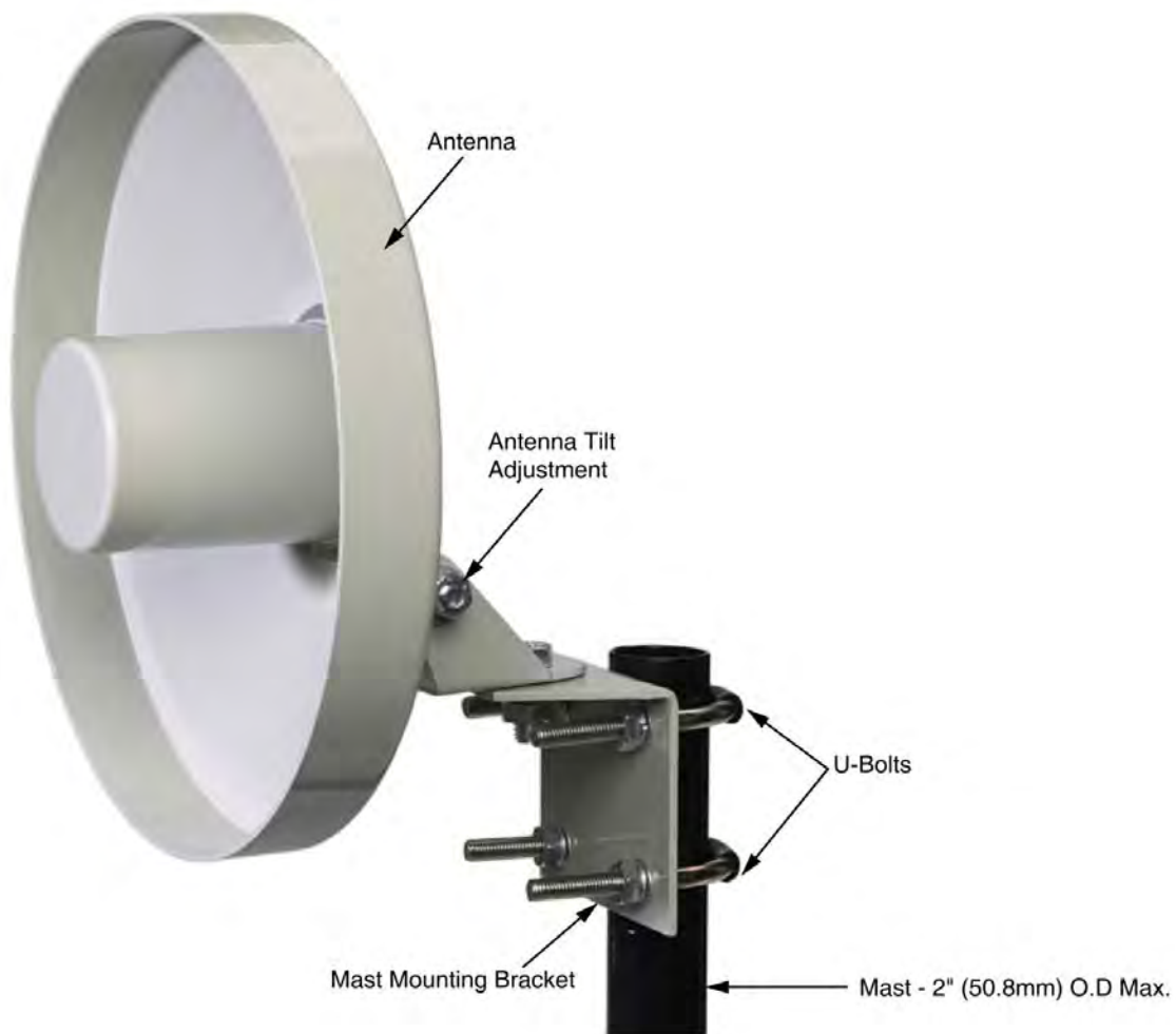
Figure 4-3 Directional antenna mounting
