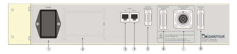
All connectors on the ULTRASTAB SATURN are placed on rear of the unit.
