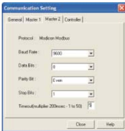
Select the appropriate communication parameters for all the ports.
