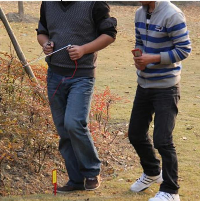
8. First walk around the Antenna and the transmitter in a ring, semi diameter is about 5-10m, to make sure a point.
