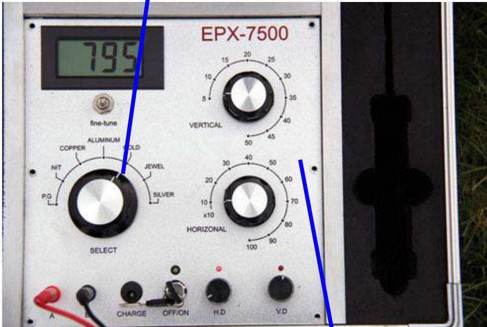
Turn Horizontal Distance Selector and Vertical Depth Selector to select the detecting range and detecting depth.
