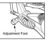
rocks slightly during use, turn one or both of the Adjustment feet under the front Stabiliser until the rocking motion is eliminated.
