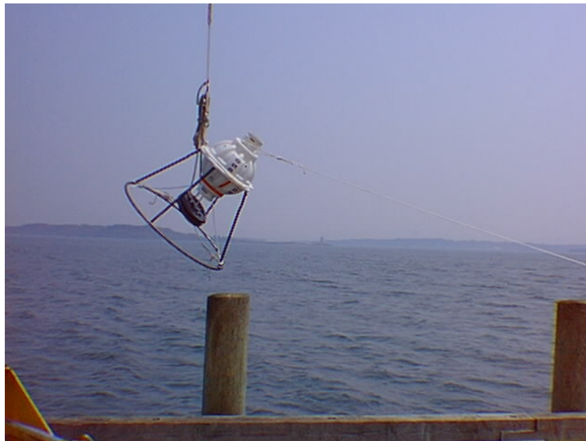
Photo 12-2 Lifting Point for C-PIES Deployment
