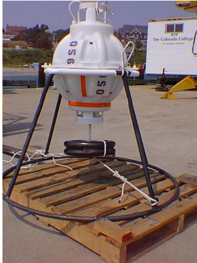
Photo 12-1 Anchor/Platform Attachment to C-PIES
